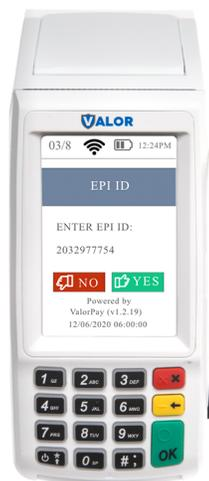
After making parameter changes, you must perform a download on the device by pressing **★ > 6 > OK** button.
